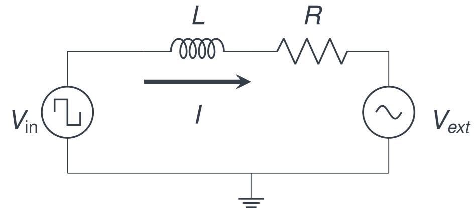
DC/AC power converters (inverters) are a component in motor control. Inverters can switch between a finite number of voltage levels to produce a load current I. The goal of this work is to bound the minimum possible energy draw  $||I||_2^2$ , which is monotonically related to the tracking error  $||I - I^*||_2^2$  and the current demand distortion of I.
